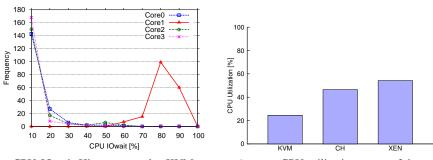
(f) Average CPU utilization among 3 hyper-(e) CPU IOwait Histogram under KVM using 4 cores; Only one core (i.e, Core1) visors. handles most of the I/O jobs.
