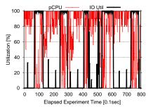
(c) Timeline of CPU and disk I/O under XEN
