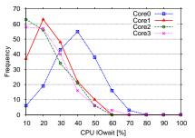
(d) CPU IOwait Histogram under CH using 4 cores; I/O jobs are distributed to all cores.
