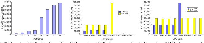
(a) Total number of LLC miss when scaling (b) Comparison of LLC misses per core be- (c) Comparison of LLC misses per core be- tween 4-core case and 5-core case; Cores tween 5-core case and 8-core case; Total used in both cases are less efficiently utilized. number of LLC miss increases 86%.
