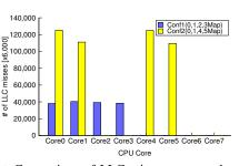
(c) Comparison of LLC misses per core between the two 4-core mappings; Cores in two different CPU packages showed overall 128% more LLC misses and the cores used in both mappings get less efficient due to significant increase in LLC misses.
