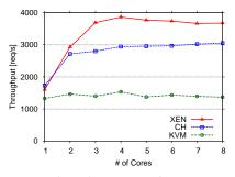
(a) Max throughput comparison among 3 hypervisors when scaling from 1 core to performance than KVM and XEN provides ing system scalability to multi-cores. up to 32% more throughput than CH.
