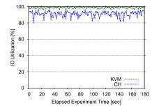
(b) Timeline of disk I/O utilization under CH and KVM configured with 4 cores; Both 8 cores; CH achieves at most 123% better cases, the disk I/O was the bottleneck limit-
