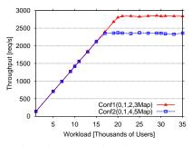
(a) Throughput comparison between the two 4-core mappings (4 cores in 1 CPU package vs 2 cores in 2 CPU packages); VMs mapped with cores in same CPU package provides 22% more performance than VMs with cores mapped to different CPU packages.
