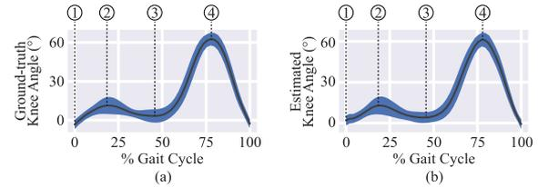
**Fig. 5.** Comparison of a) ground truth gait cycles and b) gait cycles estimated from sensor readings. The solid line is the mean knee angle and the shaded area represents one standard deviation. Four important kinematic parameters during gait are annotated in the figures: 1) the knee flexion/extension angle at the heel strike, 2) the peak flexion angle during the stance phase, 3) the knee flexion/extension angle at the toe-off, and 4) the peak flexion angle during the swing phase.
