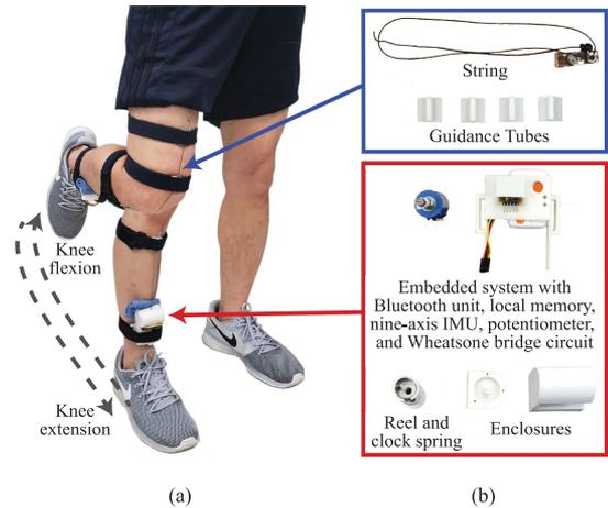
Fig. 1. (a) The final design of the proposed system at knee extension and flexion positions. (b) Individual components of the proposed system.
