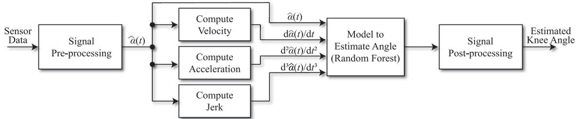
Fig. 2. The processing pipeline for estimating knee angles given potentiometer readings transmitted by the sensor. Calibration consists of recording readings at  $0^\circ$  and  $90^\circ$  knee flexion. The calibrated readings and their first three derivatives are the only inputs to the Random Forest model.
