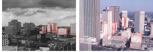
Figure 4. Time-Dependent Geometry. Scene geometry in both 1930 (left) and 1972 (right) is overlaid on two photos from their recovered 3D viewpoints. Observe that the geometry changes dramatically over the years. Our illumination estimation and color matching relies on such a time-varying scene description to accurately model shadows and establish corresponding regions across images.
