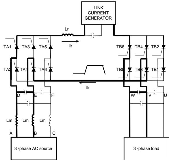
Fig. 1 USRC as a 3 phase input and 3 phase output system
