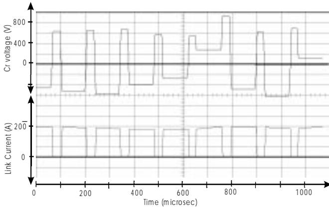
Fig. 13 Virtual test bed results : Cr capacitor voltage and link current
