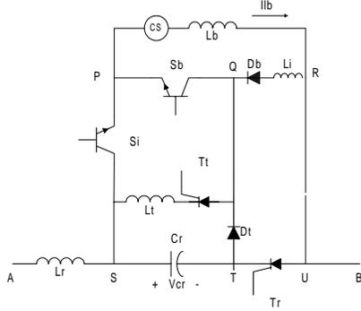
Fig. 2 Link Current Generator [1]
