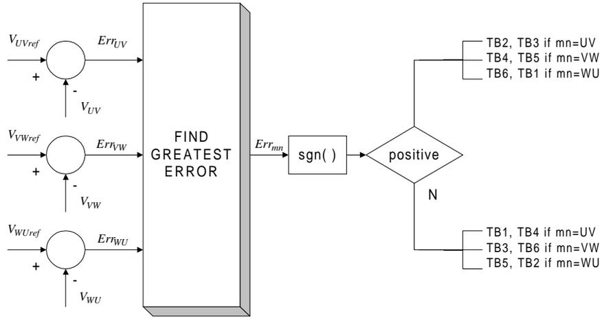
Fig. 3 Largest Error Algorithm for Output Matrix Selection
