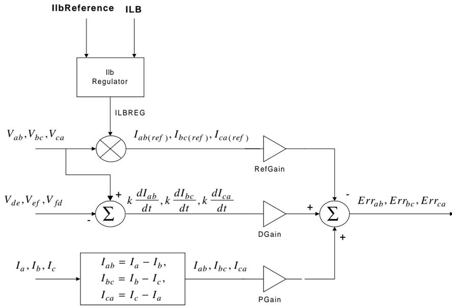
Fig. 4. Input Error calculations
