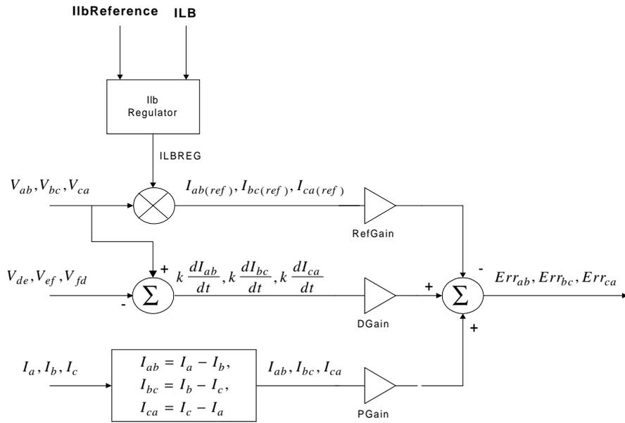
Fig. 4. Input Error calculations
