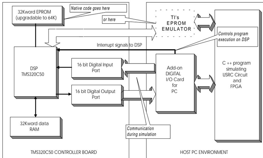
Fig. 7 Block Diagram of the Virtual Test Bed
