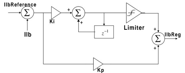
Fig. 5. Ilb PI Controller with anti-windup
