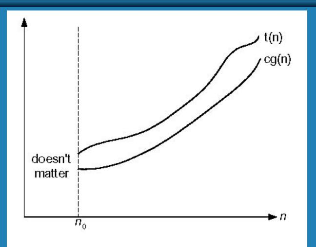
**Fig. 2.2** Big-omega notation:  $t(n) \in \Omega(g(n))$
