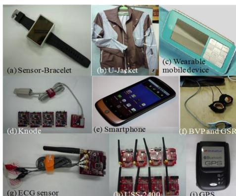
Figure 2: Smartphones and sensor devices deployed for the prototype system
